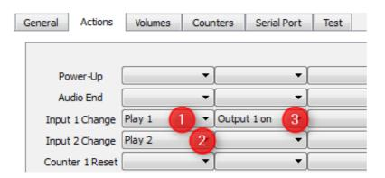
A couple of seconds later we want it to be turned off again. This delay is implemented using counters. Such a counter gets an initial value from where it is continuously counted down. This can either be done automatically by a 0.1- or 10 second clock or manually by executing the action **Counter Decrement**. When a counter reaches 0, the event **Counter Reset** is triggered.
